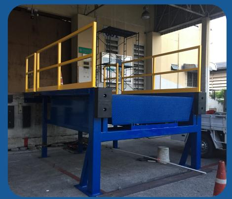
The Free Standing Mount Dock Leveller is suitable for loading bays where a concrete pit cannot be constructed. It consists of two parts: the dock leveller itself and the free-standing frame that supports it. This configuration requires more installation space, as additional area is needed to accommodate the free-standing structure.
